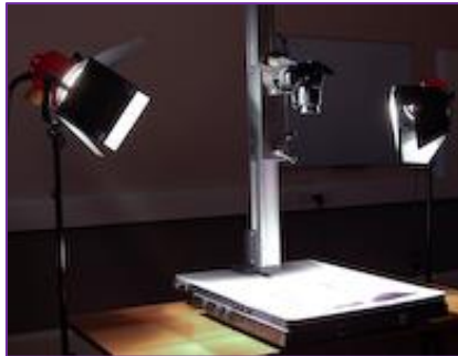
Figure 2: Camera mounted on copystand, separate lights positioned either side
